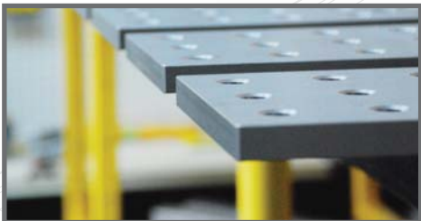
Plates edges overhang provide clamping surfaces all around the table.
